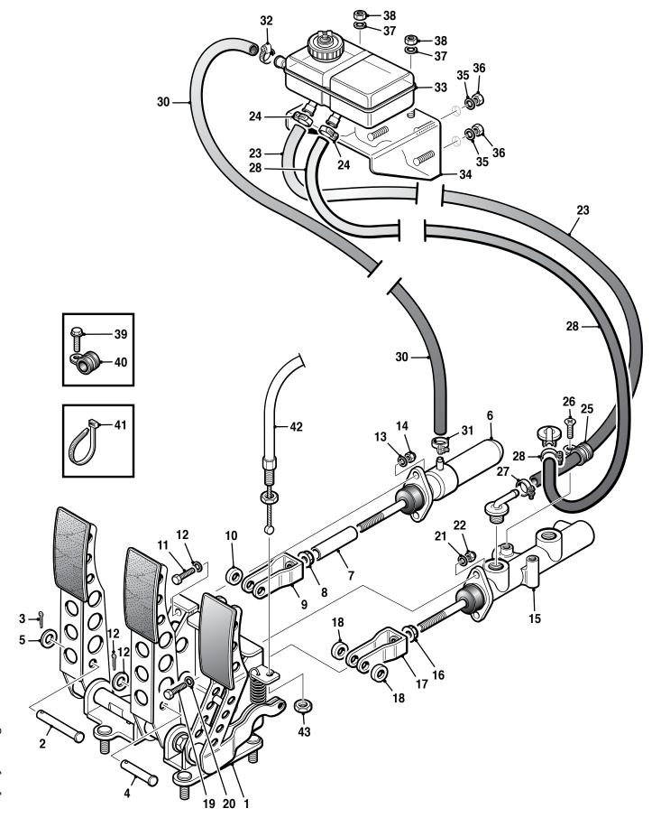
Pedal Box (????? 2012 onwards) and Hydraulics
